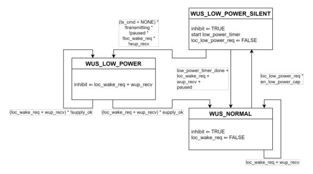
Figure 8-2--PHY power mode state diagram
