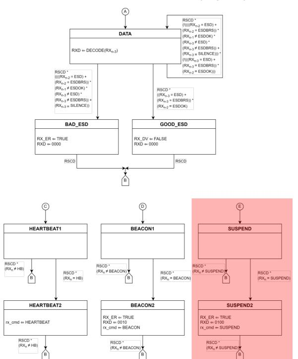
Figure 147-8--PCS Receive state diagram, part b
