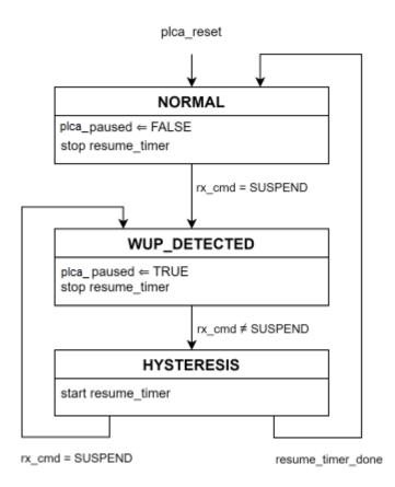
Figure 148-8--PLCA Pause state diagram
