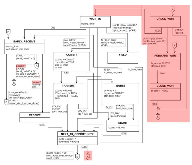
Figure 148-4--PLCA Control state diagram, part b
