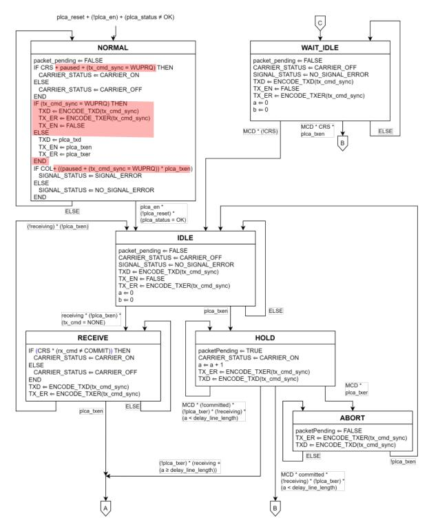
Figure 148-5—PLCA Data state diagram, part a
