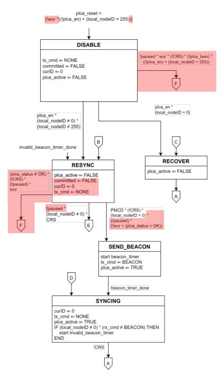
Figure 148-3--PLCA Control state diagram, part a
